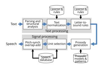
Figure 1: Overall architecture of the TTS engine
