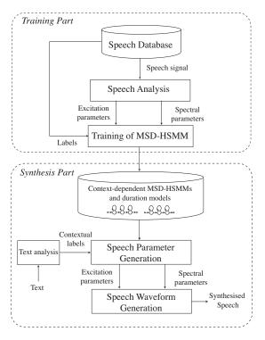
Figure 1: General block diagram of the HTS system.
