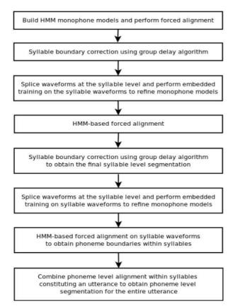
Figure 3: Flowchart of hybrid segmentation
